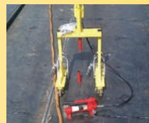
Stiff Jack (6,000 lbs/2,700kg holding force; steel frame)
